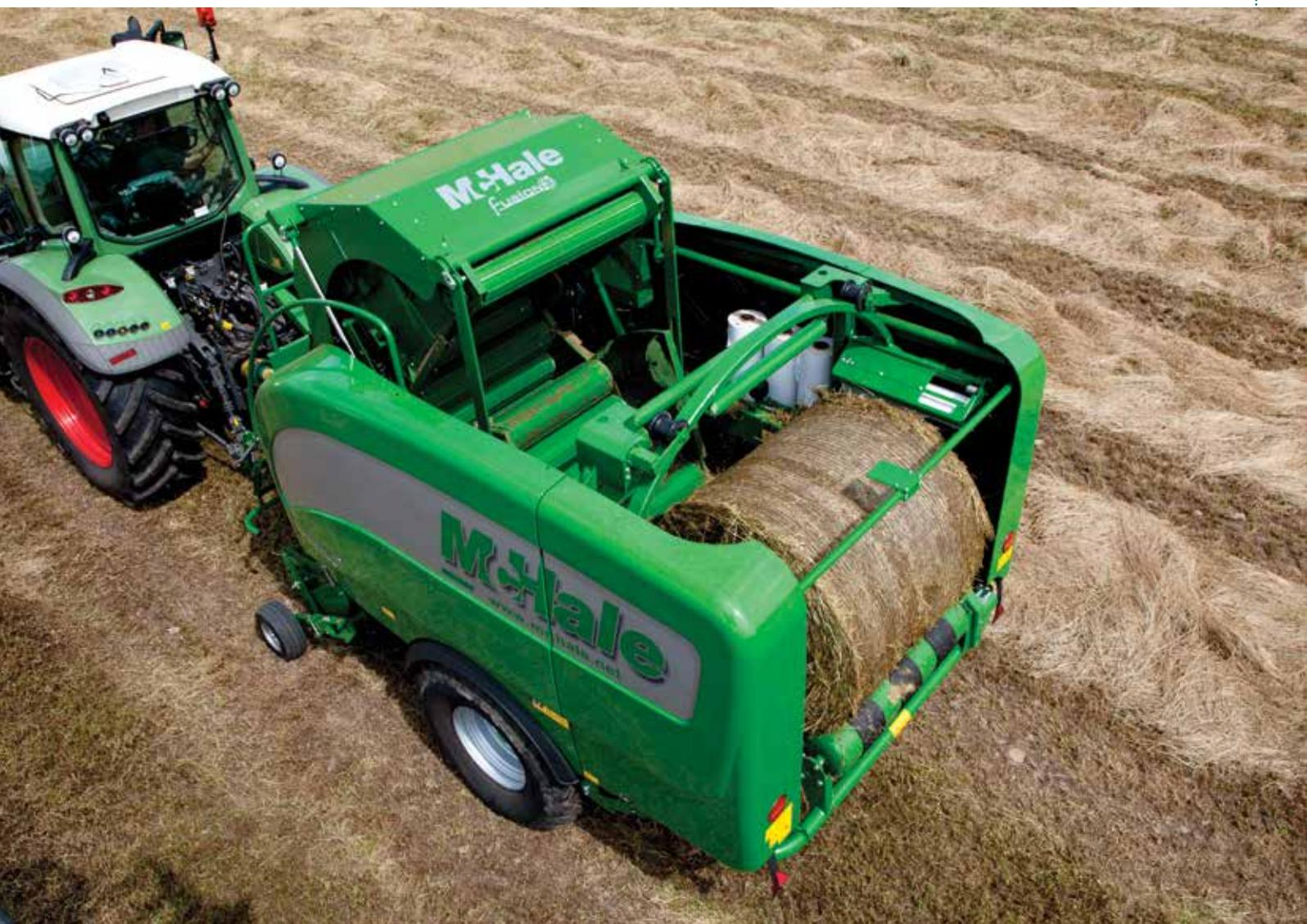
**THE MCHALE FUSION 3** is a robust, fully automatic, integrated baler wrapper recognised worldwide for its unique patented bale transfer, vertical wrapping ring and high output. The machine is equipped with a 25-knife chopping unit, automatic progressive greasing system and a servo operated load sensing control valve, which when combined with the Expert Plus control console, makes the baling and wrapping process fully automatic. The machine is fitted with 560/60-22.5 tyres as standard.
