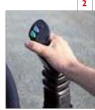
I- Control valve with direct control (for CI and CIs loaders)
