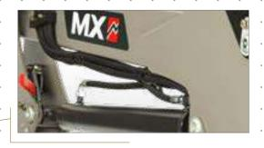
The hydraulic lines and polyurethane cable array pass discreetly along the underside of the loader arms. This protection ensures that they remain clean and easy to access.
