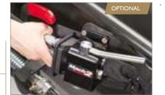
Instant multi-coupling for loader/implement hydraulics with the MACH 2® connector.
