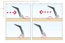
The dumping rams are linked to a double pressure limiter, also known as an anti-impact valve, which protects the loader in both forwards and reverse (scraping) motion.
