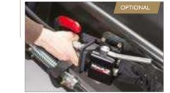
Instant multi-coupling for loader/ implement hydraulics with the MACH 2® connector. page 50
