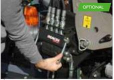
coupling of tractor to loader hydraulic > page 50 and electric lines \*
