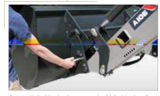
Automatic locking implement carrier. Unlocking handles accessible from each side of the frame.
