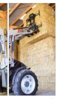
Hydraulics necessary: I function • Minimum front loader lift height: 3.60 m pivot • Equivalent or greater power
