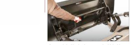
Automatic locking implement carrier. Unlocking handles accessible from each side of the frame.
