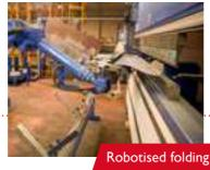
Fully-automated line with a folding capacity of 320 tonnes over 4 metres.
