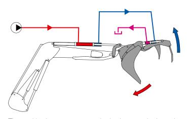
The combined movements are maintained at an optimal speed thanks to an exclusive concept that reuses the oil returned from dumping to fuel the 3rd function, with no loss of flow.
