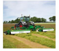
The Pro Glide range of rear mowers are fitted with patented ground adaption technology, which allows the bed to move back and up if the bed encounters small obstacles. This results in higher mowing speeds being able to be achieved without the interruption of having to reset the break back.
