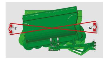
The Pro Glide range of rear mowers are fitted with patented ground adaption technology, which allows the bed to move back and up if the bed encounters small obstacles. This saves time and maximises throughput as it means the obstacle does not trigger the main break back protection. This results in higher mowing speeds being able to be achieved without the interruption of having to reset the break back.
