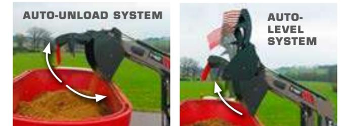
The AUTO-UNLOAD System allows a load to be emptied by opening the grab and tipping the bucket at the same time. The AUTO-LEVEL System then automatically returns the bucket to the horizontal position.
