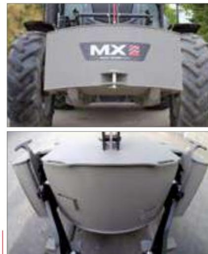
All MULTIMASS have a steel fabricated structure with **yoke hitching points** for high impact resistance and durability.
