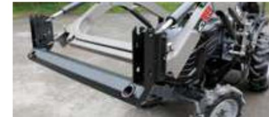
With this optional implement carrier, changing implements could not be simpler using straightforward manual pinning. It is capable of holding two MANUBAL spikes, or even TRC500 tines for handling your pallets.
