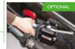
Instant multi-coupling for loader/implement hydraulics with the MACH 2® connector. [page 50](#)
