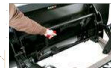
Automatic locking implement carrier. Externally accessible release handle.
