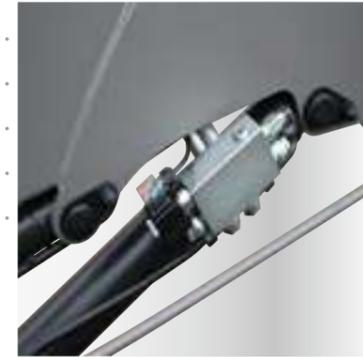
Lifting/dumping safety device
