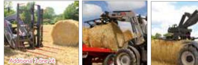
Hydraulics necessary: 1 function • Minimum front loader lift height: 3.60 m pivot • Equivalent or greater power than the MX U410/T410.
