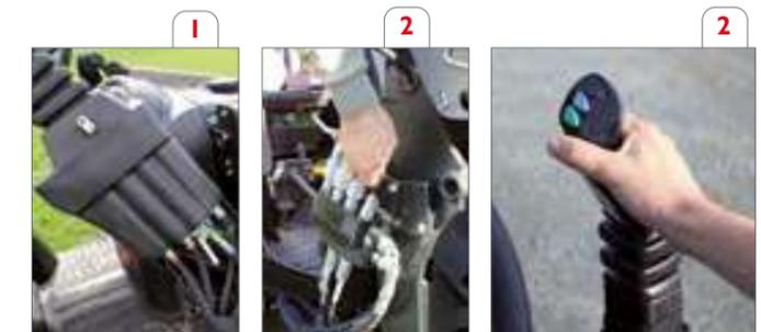
1- Control valve with direct control (for C1 and C1s loaders)
