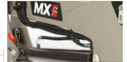
The hydraulic lines and polyurethane cable array pass discreetly along the underside of the loader arms. This protection ensures that they remain clean and easy to access.
