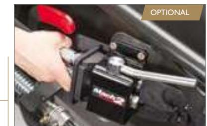
Instant multi-coupling for loader/implement hydraulics with the MACH 2® connector.
