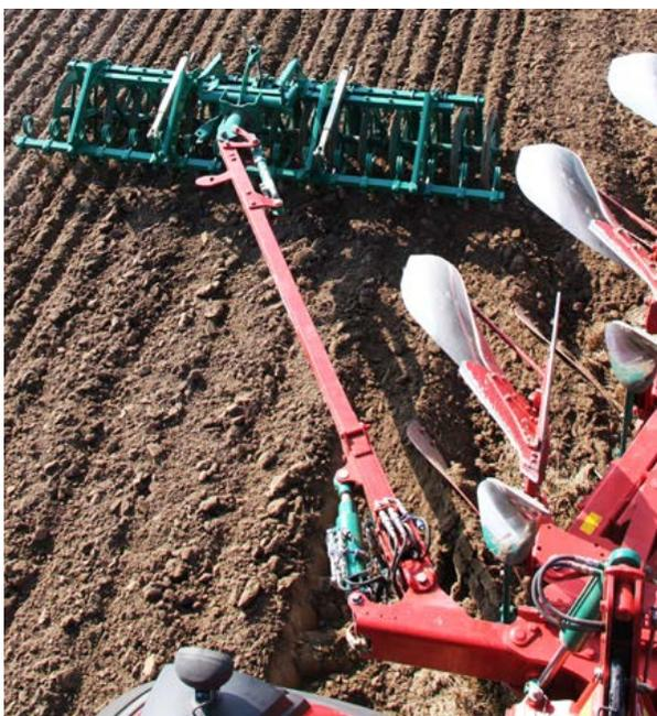
Packomat works in all ploughing conditions. It levels, re-consolidates, crushes clods, prepares seed beds, from light-dry to heavy-wet soils.
