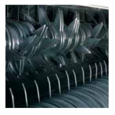
Improved silage quality The 1.40m wide cutting rotor with fifteen three-lobe double fingers positively transfers the crop to the bale chamber. With the CropCutter<sup>™</sup> system engaged, bale density is increased and silage quality improved.
