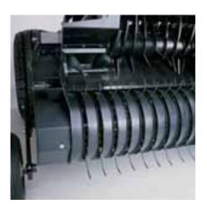
**Optimum crop transfer** The long pick-up tine guards and two short side augers ensure a smooth, uninterrupted crop flow to the feeder.
